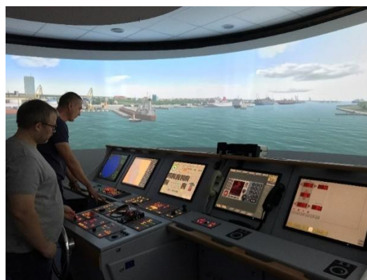
Fig. 17. NTPRO 5000 navigational simulator for Ro-Pax ship model
